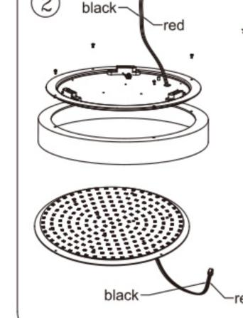
\*In the case of duo color temperature, if red wire is connected to positive pole and black wire is connected to negative pole, led chip of a kind of color temperature will be activated. If red wire is connected to negative pole, black wire is connected to positive pole, led chip of another color temperature will be activated.
